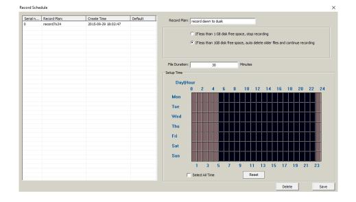
Enter a descriptive record plan name into the "Record Plan" field in the upper right area.
